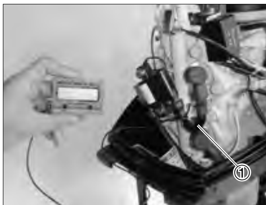
⑪ High Tension Cable
